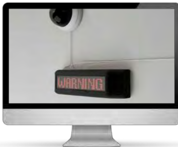
A RAM unit mounted under a legacy security camera displaying a warning message on its front panel after detecting an unusual incident.
